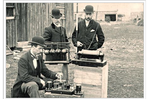
British Post Office engineers inspect Guglielmo Marconi's wireless telegraphy (radio) equipment in 1897.
