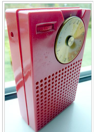
The Regency TR-1 which used Texas Instruments' NPN transistors was the world's first commercially produced transistor radio.
