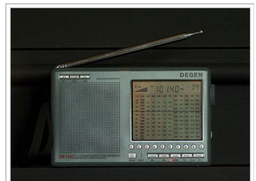
Degen DE1103, an advanced world mini-receiver with single sideband modulation and dual conversion
